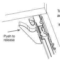
To remove the drawer, open and locate the clips on each side of the drawer base. squeeze both clips and pull the drawer forward while lifting to remove.
