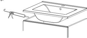
We recommend that you read the sealant packaging for the curing time. Do not use until the sealant is set.
