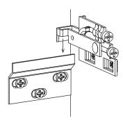
Gently lift the cabinet into position so that the cabinet hangers sit onto the wall brackets. Make sure that the cabinet is securely held in place before letting go.
